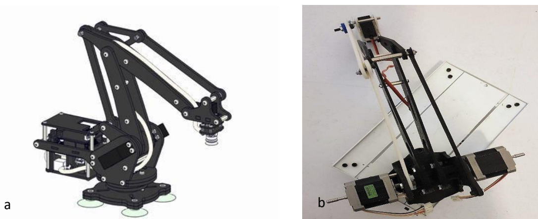
Figure 2.: uArm manipulator (a), Our manipulator (b)
